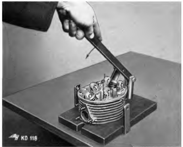
15 Dismantling cylinder head
