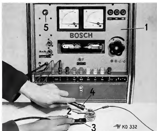
43 Check contact breaker for short-circuit to earth
